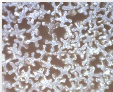
Nexstar Ribbed Cross Section fibers are well formed, will carry more paint due to their shape and low packing density and will be economical to use as they are lighter. They also flag and wear better than the mini-hole.
