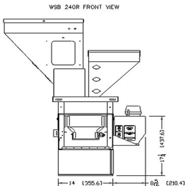
Dry raw material is conveyed to individual air tight hoppers from where a computer weighs the components of each batch, mixes them with a rotary cylinder and makes the blend available to the hopper mounted on the throat of the extruder.
