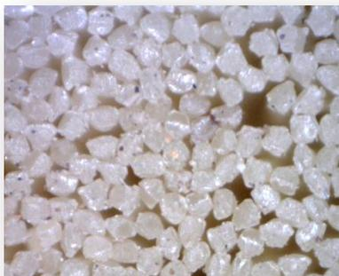
A typical Mini Hollow Cross Section. Most fibers have solidified and the 'hole' has disappeared.
