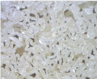
A typical Hollow Cross Section. Most fibers are crushed and have not fused. Brushes made from such fibers will quickly deteriorate.
