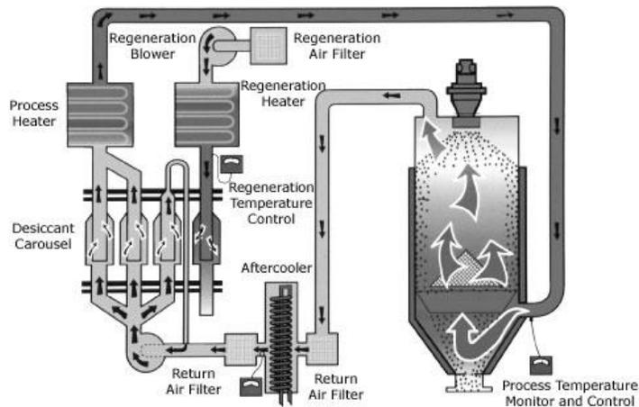
Air is heated inside a hopper which flows through the granules stored inside, carrying moisture with it. This air is then routed through a carousel containing desiccant beads which trap the moisture. The cycle is repeated until the desiccant is full of moisture and ceases to function effectively. The air path is then changed and a second carousel becomes active while the first is regenerating.
