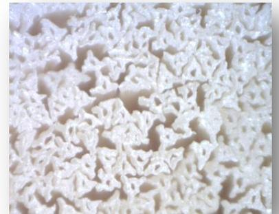
Nexstar Spoked Cross Section has a well defined mini-hole and fins like ribbed. This special cross section will allow the fabrication of more robust brushes as compared to hollow at a marginal cost increment.
