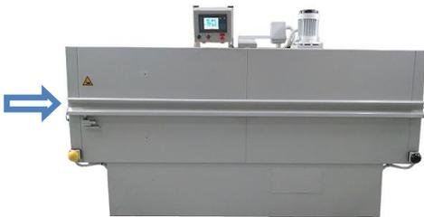
Annealing stabilises the molecular structure of the fibers by relaxing them. Properly annealed fibers will not bend or curl under normal circumstances. Fibers can be annealed inline during the extrusion process by passing them through a hot air oven (arrow mark on the picture) or post extrusion i.e. by winding a lot of fibers on a jig and placing them in an oven.
