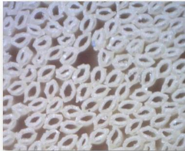
Nexstar Hollow - all the fibers are properly fused and not crushed. Such a fiber will have better bend recovery, will carry more paint and is economical as its lighter.
