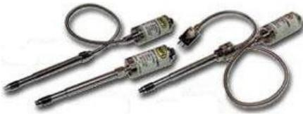
The second step is the inclusion of 3 precision melt pressure transmitters which will keep both the extruder output and melt viscosity constant by calculating delta P and sending signals to a Logic Controller/Frequency Drive which in turn will control the RPMs of the extruder by changing its revolutions depending on delta P. Once the operator sets the desired pressure in PSI, the extruder runs in auto mode and no manual adjustments are necessary.
